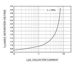
Figure 3. Collector-Emitter Saturation Voltage
