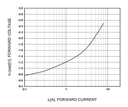
Figure 4. Damper Diode Forward Voltage
