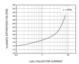
Figure 2. Base-Emitter Saturation Voltage
